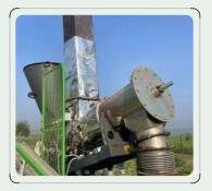
TAKACHAR'S PROTOTYPE, THE "TAKAVATOR," A PORTABLE MACHINE THAT TURNS CROP WASTE INTO BIOFUELS, CARBON-BASED FERTILIZER BLENDS, AND OTHER VALUABLE BIOPRODUCTS
